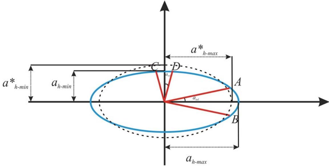
**Figure 1** True Anisotropic ellipse (solid) and the estimated anisotropic ellipse (dashed) in 2D case when there is no bandwidth
