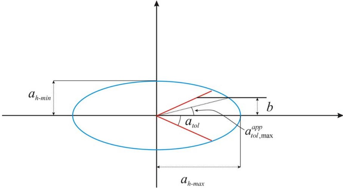
**Figure 2** Anisotropic ellipse in 2D case with bandwidth for maximum direction of continuity
